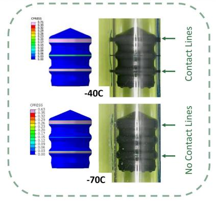
Stopper imaging at target temperatures supports CO<sub>2</sub> ingress results
