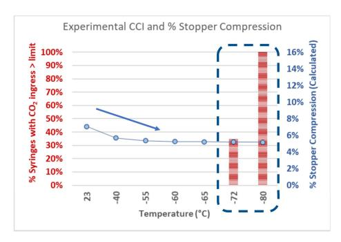
% Stopper compression reduces with temperature but is still theoretically adequate even down to -80C
